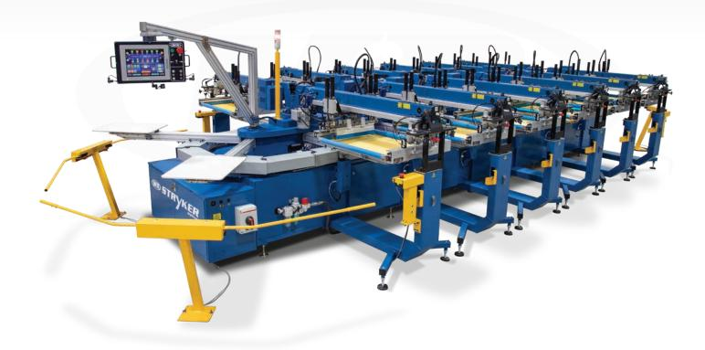
M&R's Stryker sets the standard for oval format screen printing presses. Its oval design takes up less floor space than comparable carousel automatic screen printing presses, making more efficient use of the available production area. Available in three print format sizes and expandable from 10 to 52 stations with selectable printhead locations, the Stryker can be tailored to almost any production requirement, floor layout or shop size.
