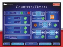
Digital display tracks production and makes it easy to manage process elements like Index Dwell, Preheat Mode, Flash Duration, and Flash Delay.
