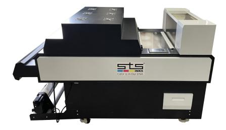
After the STS 628D prints your design, our **Automatic TPU Adhesive Powder Shaker** takes over by evenly spreading, then melting the exact amount of adhesive material directly onto your design saving time, effort and cost. Three resources you need to conserve to run a profitable business. Also, with a handy vacuum absorption platform and infrared heat drying, you are assured a smooth result every time.
